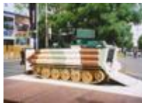
M113 APC fitted with ASPRO-H armour package, RAFAEL Remote Control Weapon Station armed with a cannon and ASPRO-A-L (Trophy Light) showing antenna mounted either side above hull rear. (Christopher F Foss)
