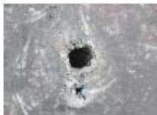
Close-up of the penetration achieved by the Spike-LR warhead. (Source: Grzegorz Holdanowicz)
