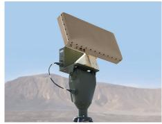
The RF sensor rapidly scans the environment, detecting and identifying potential threats in the area of interest. Upon detection, the system classifies the threat, alerts the user and enables various mitigation actions to neutralize the threat.
